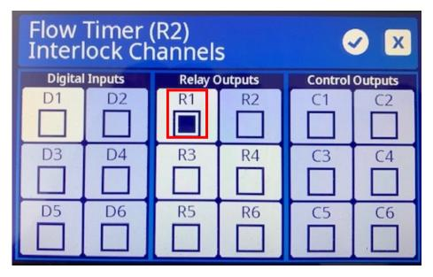
Since the R1 menu has Interlock Channels R2, and the R2 menu has Interlock Channels R1, whichever relay activates first will prevent the other relay from activating. This is referred to as Mutual Interlock.
